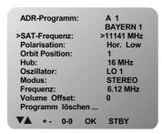
The menu entries "Programme name" and "De-emphasis" are dropped. With digital radio programmes, the broadcasting station includes the programme name in the transmission.
